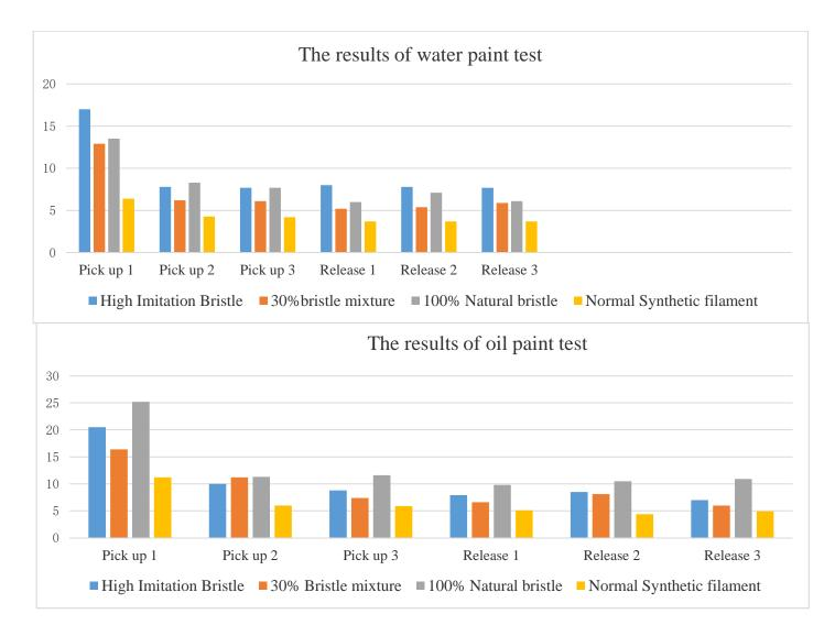
All tests were carried out under the same conditions 2 inch Flat Paint Brush
